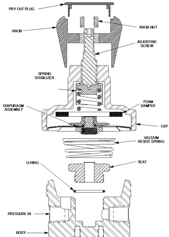
15. Place a small amount of Krytox or other lubricant on the outer threads of the body if the regulator body is steel. Do not apply lubricant to threads if regulator body is brass.
