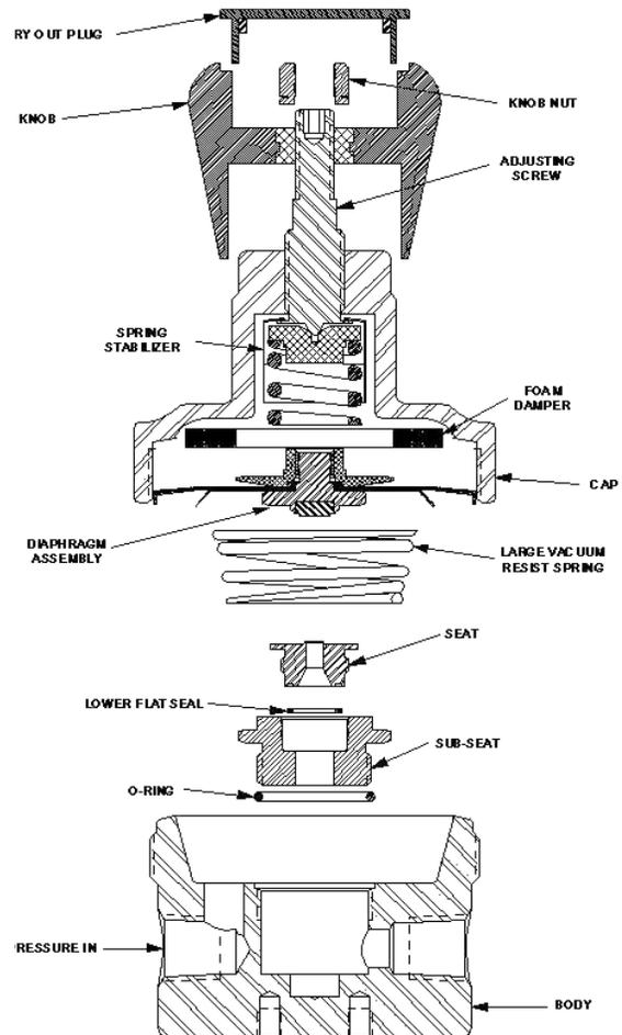
19. Finish tightening seat to 25 lbf•ft (34 N•m). (15 lbf•ft (20 N•m) for brass body).
