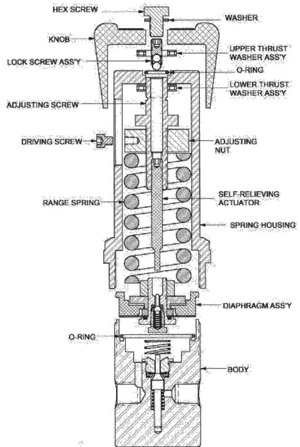
12. Turn the adjusting screw clockwise until the outlet gauge reads a pressure equal to 100% of the maximum rated pressure range for this unit. Put more foam around the slot in the spring housing. If any leaks are present, immediately turn the adjusting screw counter-clockwise to relieve the outlet pressure and search for the cause of leakage.
