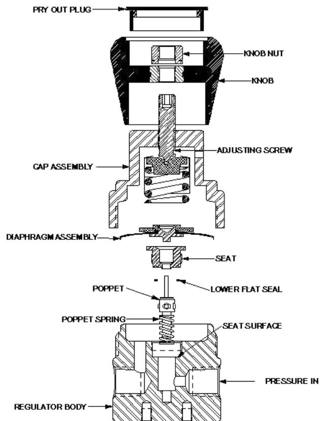
21. Place new diaphragm assembly onto regulator cavity.
