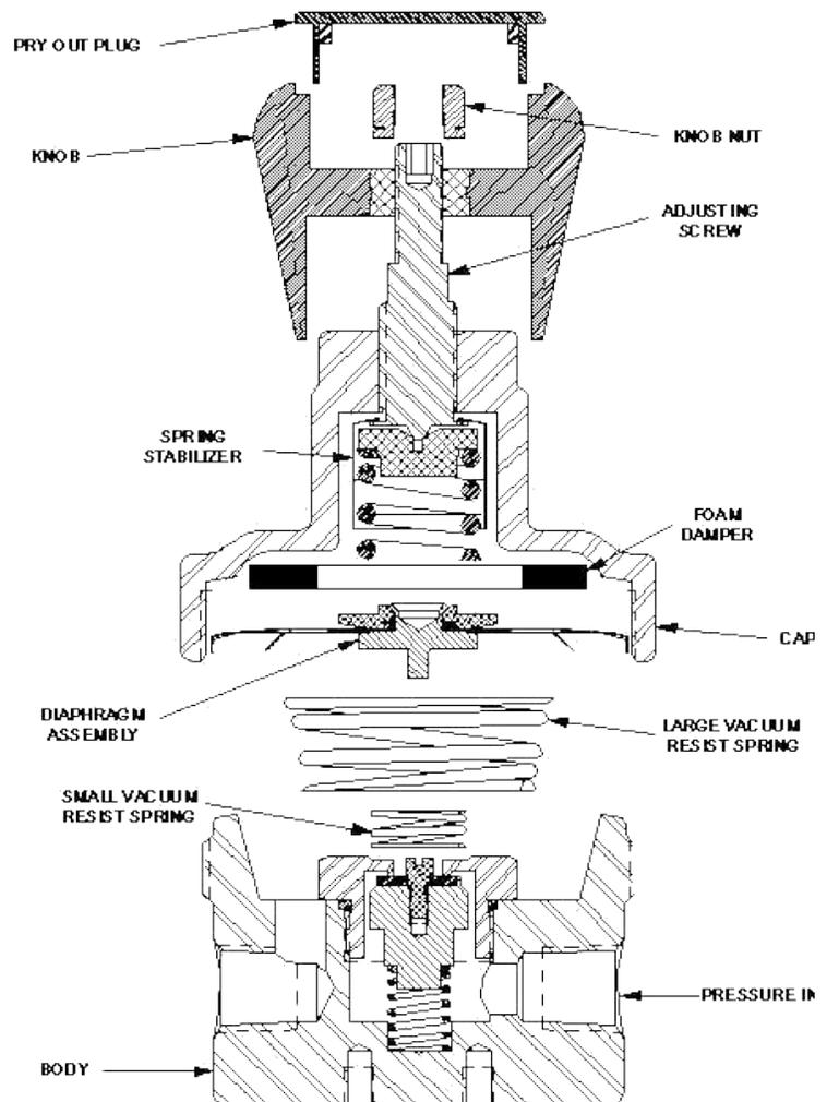
11. Finish tightening cap to 60 lbf·ft (81 N·m). (40 lbf·ft (54 N·m) with teflon / viton diaphragm). Attach a pressure gauge and quarter-turn valve to the outlet port. Leave the valve in the open position.
