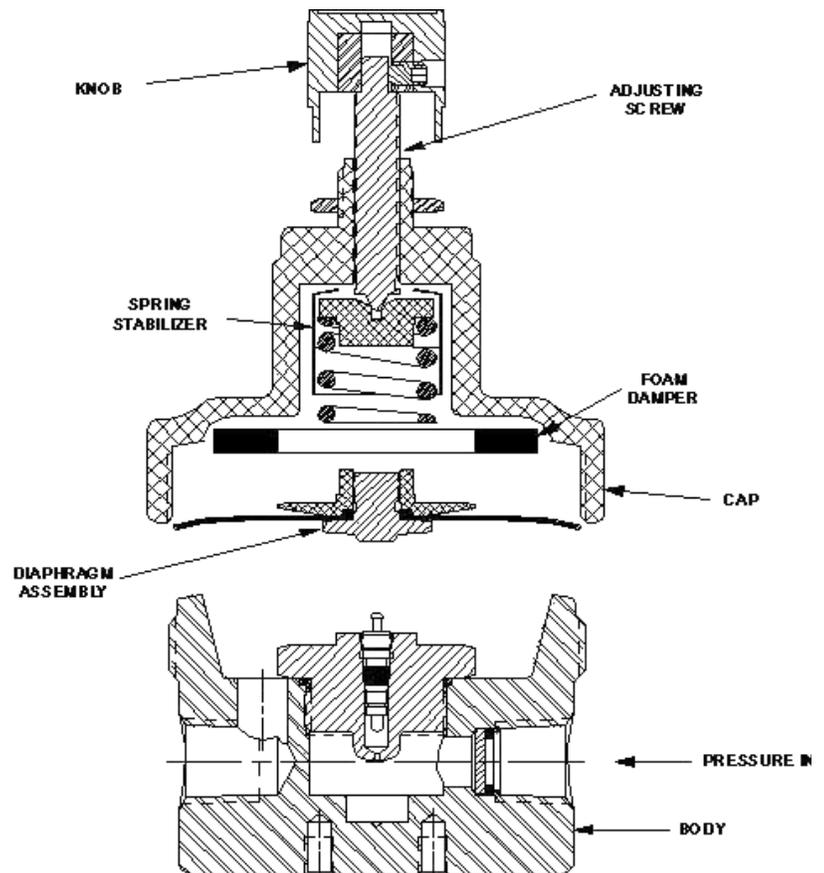
14. Squirt a leak detecting fluid around the base of the cap where it meets the body. Agitate the fluid to form foam and apply around the 0.125 (3.1mm) leak detection port in the bonnet of the cap.
