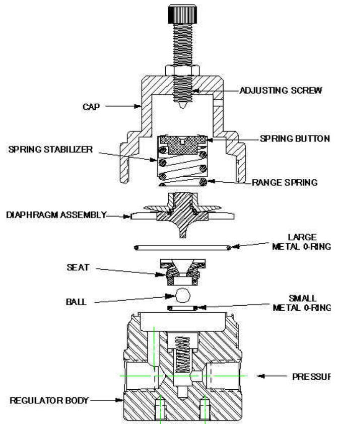
21. Place new metal o-ring in the groove on the nose of the body.
