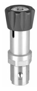
To meet the demands for the safe reduction of inlet pressures up to 15,000 psig, GO Regulator has designed the PR-58 Series regulator. This precision regulator features a piston sensing design which provides the operator with low adjusting torque requirements when setting the outlet pressure. The body is constructed from 316L stainless steel, providing the ultimate in safety and corrosion resistance.
