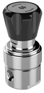
The PR-15 Series is a versatile pressure reducing regulator designed to meet the demands for outlet pressures up to 3000 psig while maintaining superior corrosion resistance in a compact package. This regulator features a piston sensing design which is provides the operator with low adjusting torque when setting the outlet pressure and has an optional T-handle for easy adjustment in the field.
